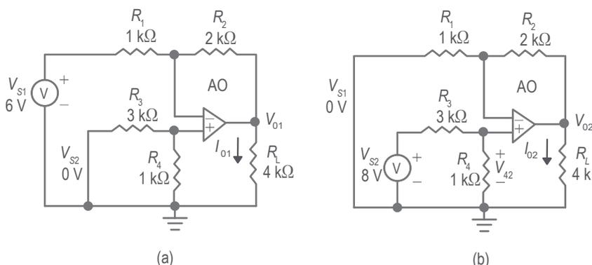
**Figura 6.** Circuito con: (a).  $V_{S1} = 6 \text{ V}$  y  $V_{S2} = 0$ ; (b).  $V_{S1} = 0 \text{ V}$  y  $V_{S2} = 8 \text{ V}$ .
