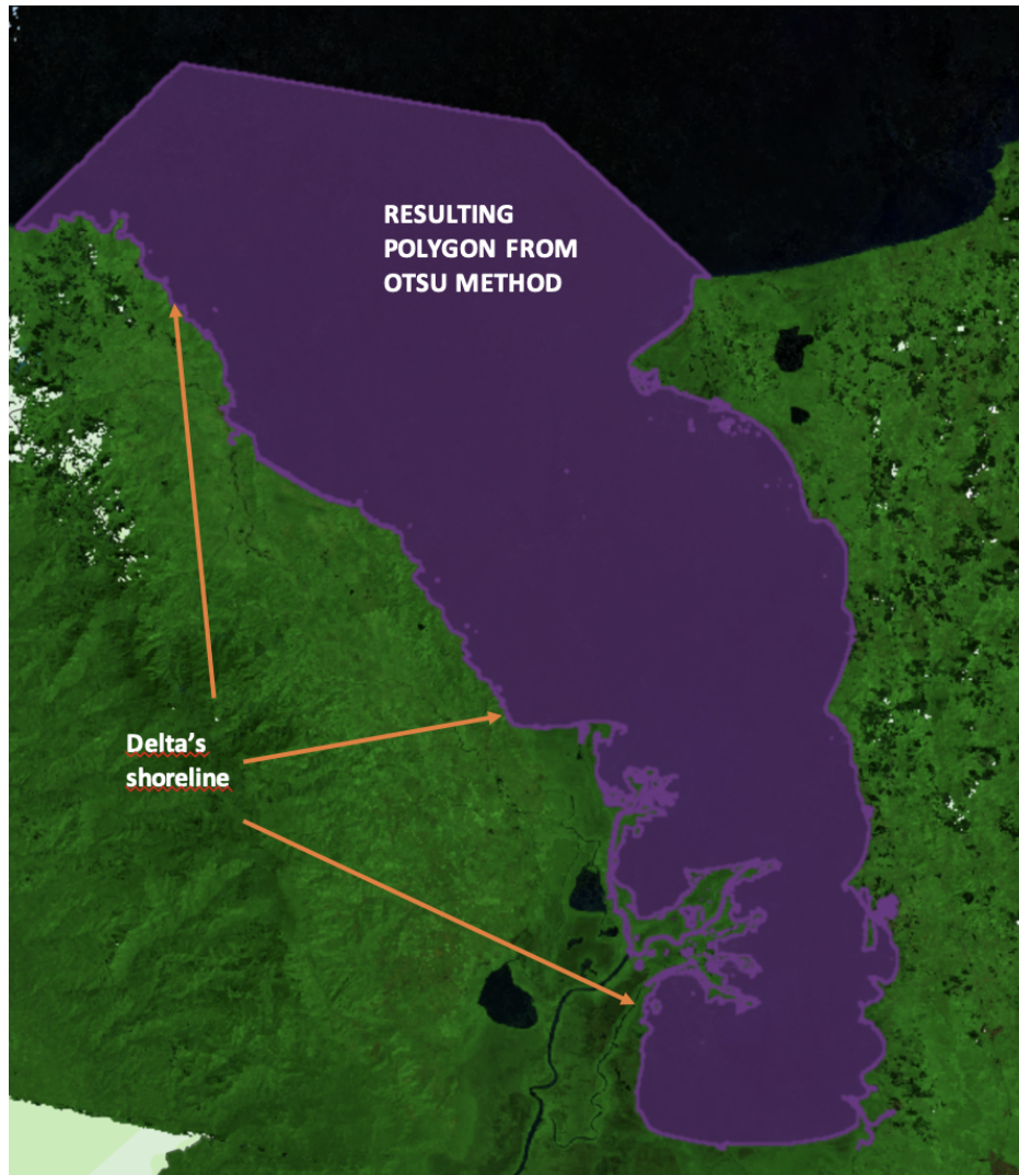
Figure 8. Polygon obtained after applied Otsu method, one of its sides is the shoreline of the delta
