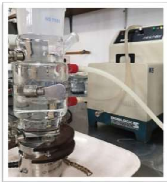
741 Fig. 9. Ultrasound reactor used for experiments.
