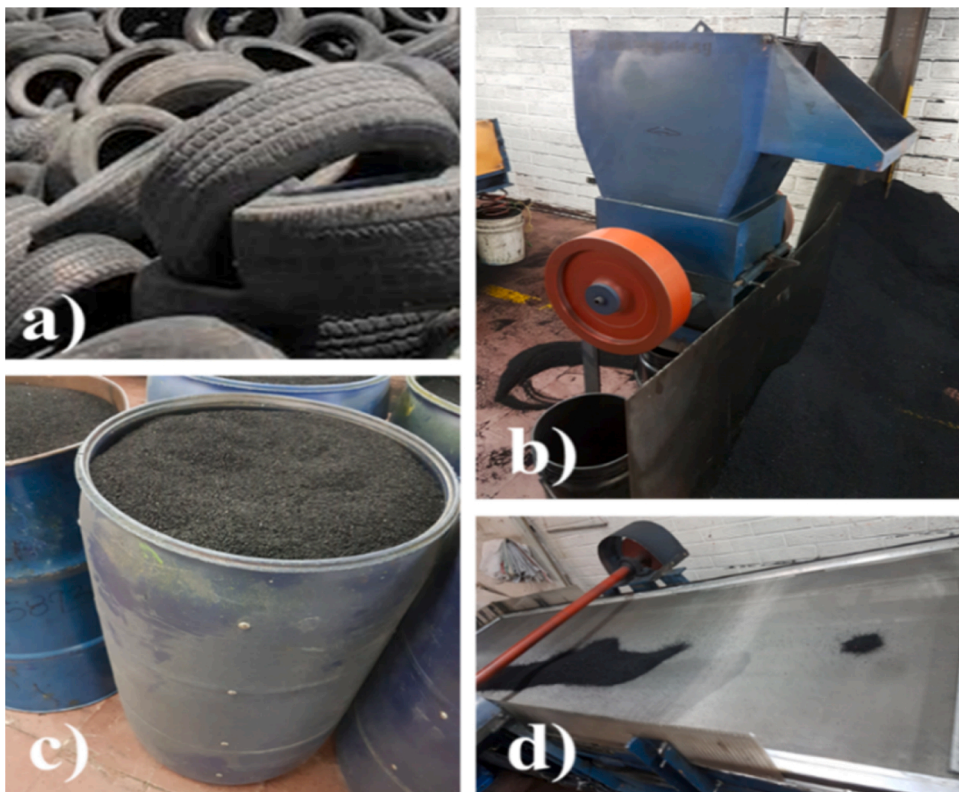
Fig. 1. Rubber grinding process. a) Car tire waste, b) grinding, c) 30 mesh ground rubber, and d) industrial linear vibrating sieve shaker.
