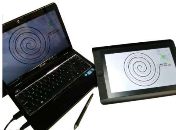
Figure 3.3: System to capture handwriting data
