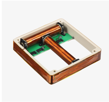
Fig. 1. Magnetorquer for CubeSat. Source: [9].
