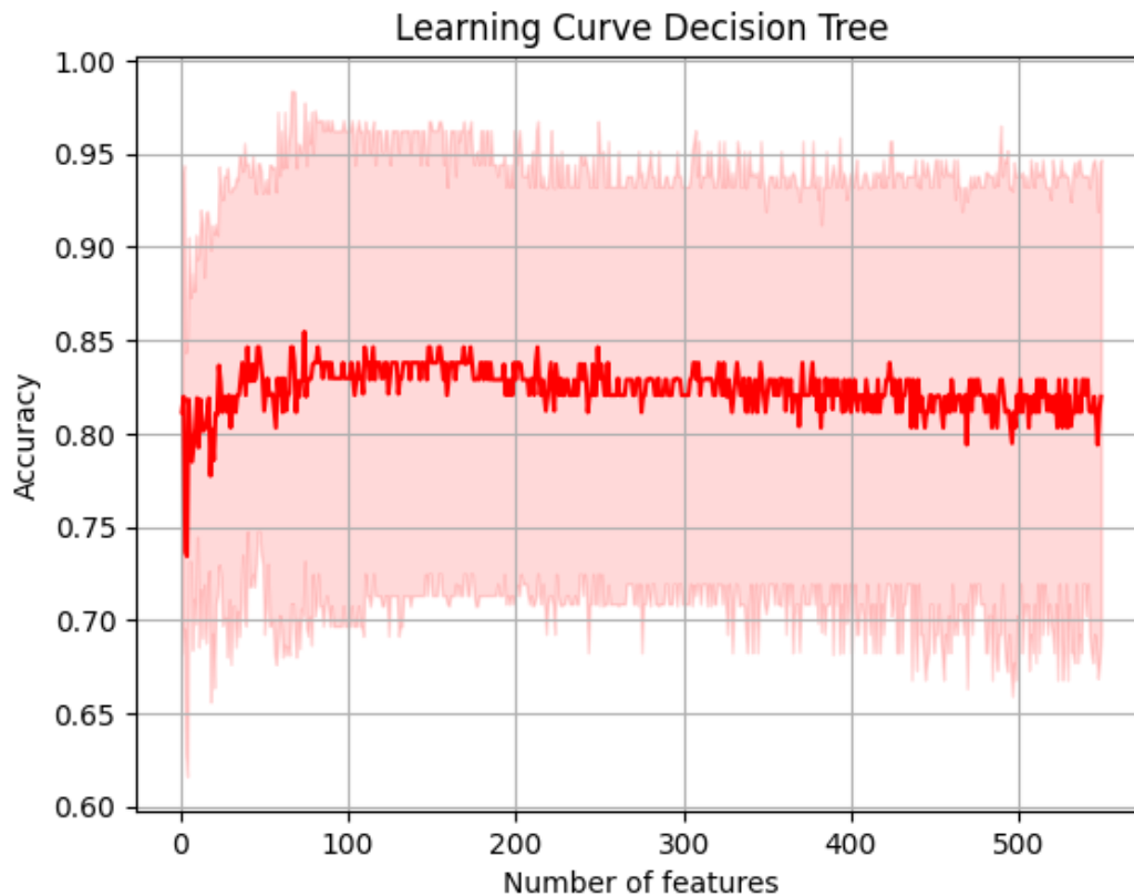
Figure 41 Relationship between the number of features and the accuracy of the model without neuroHarmonize
