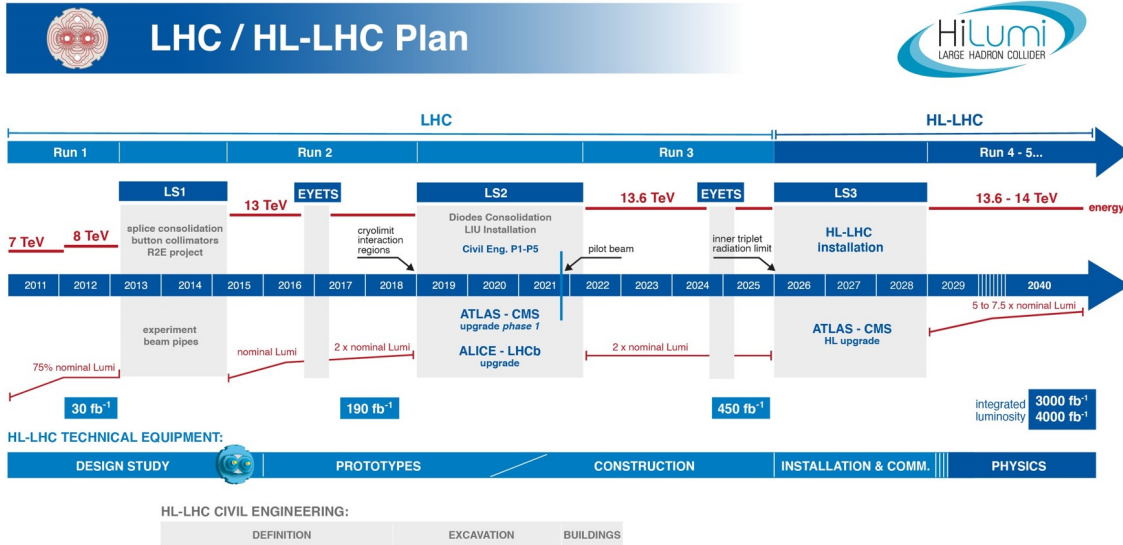
Figure 1.6: HL-LHC planned upgrade schedule, taken from [18]. The most updated one can be always consulted in [19]
