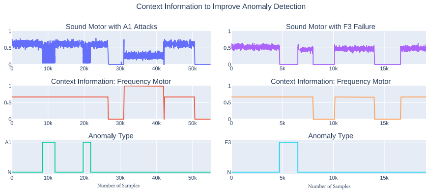
Fig. 11. Context information. By incorporating motor data into the Industrial Internet of Things (IIoT) dataset, it becomes possible to distinguish between normal and abnormal behavior.
