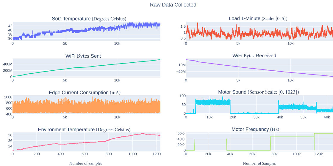
Fig. 4. Raw data collected. The plots display the appearance of some of the signals that are gathered by the IIoT system.
