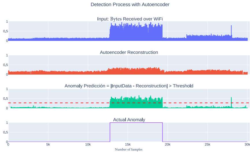
Fig. 7. Anomaly prediction with Autoencoder. Any sample above the threshold value is labeled as an anomaly.
