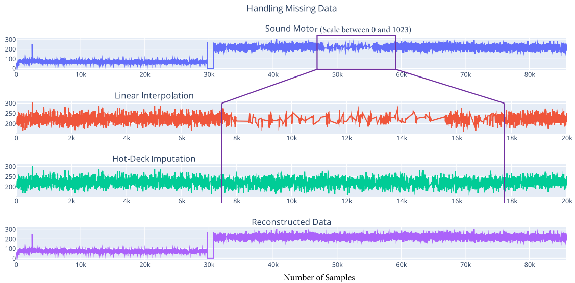
Fig. 5. Handling missing data. Two methods to replace missing values are linear interpolation, which creates a new value between two samples, and hot deck imputation, which copies a range of data from the same series.
