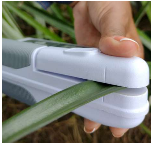
Figure 5.12: Procedure for measuring chlorophyll content using the SPAD-502 Plus instrument. Source: Own image of the development of the experimental design.
