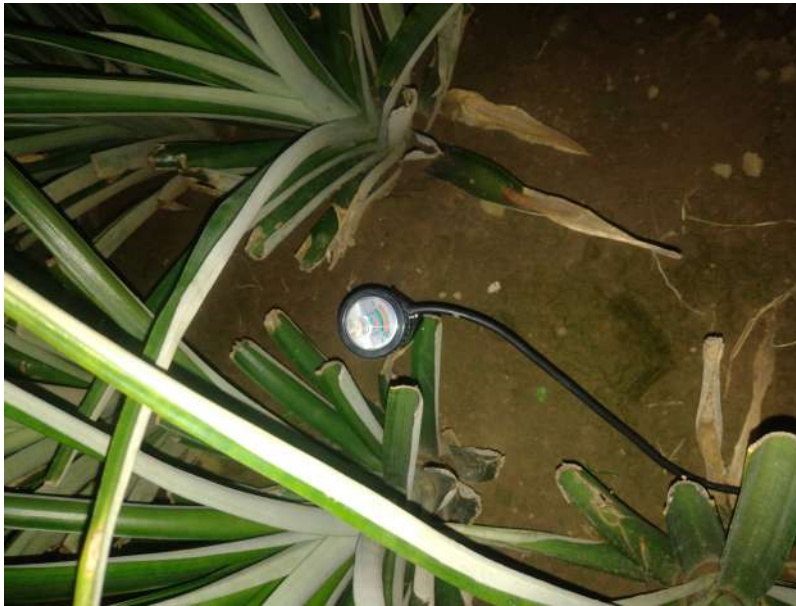
Figure 5.6: Analog pH and soil moisture sensor, this sensor was conditioned to transmit the signal to the agrometeorological station. Source: own image taken from the agrometeorological station developed for this doctoral thesis.
