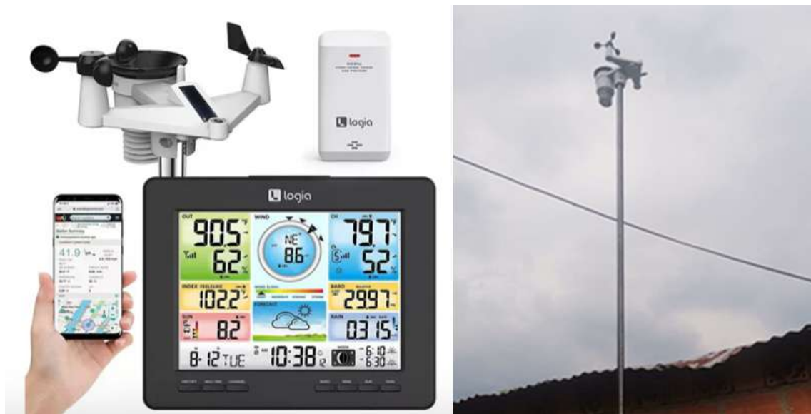
Figure 5.4: Logia Wi-fi Weather Station: 7 in 1 installed in the crop for acquisition of environmental variables. Source: left image taken from amazon.com. Right image: own image of the equipment used in the development of the experimental design.
