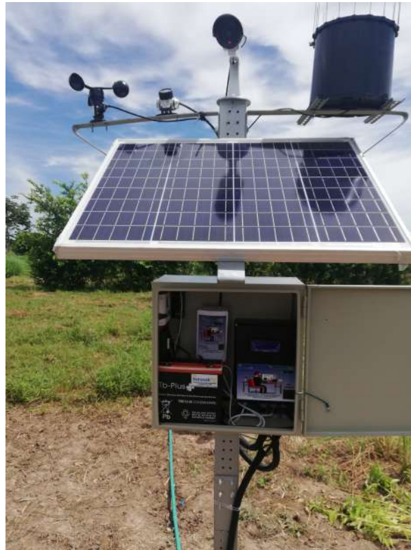
Figure 5.5: IoT agrometeorological station designed and developed for this project. It records information on environmental variables and ecological factors. Source: own image taken from the agrometeorological station developed for this doctoral thesis.
