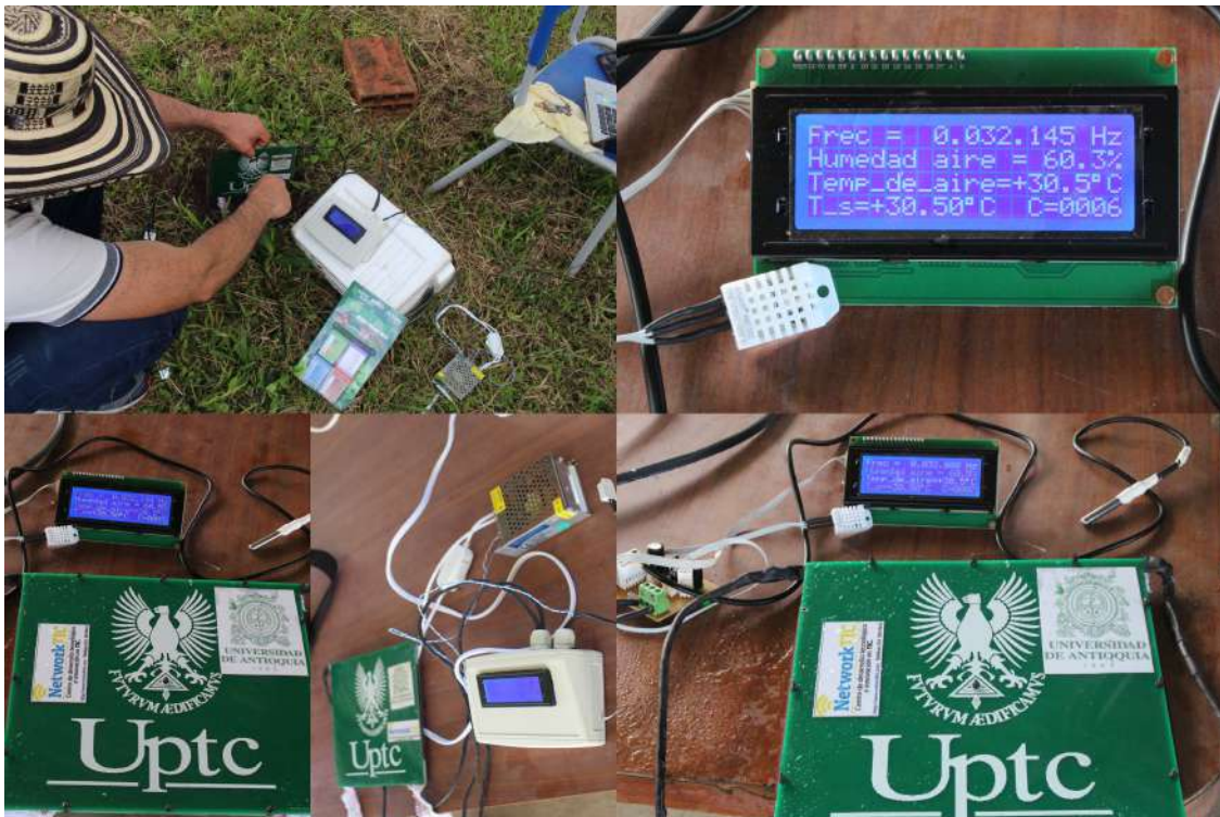
Figure 5.10: Images of the sensor and data log for the calculation of the permittivity of the capacitor dielectric material. Source: Own image of the tests performed on the parallel plate sensor.
