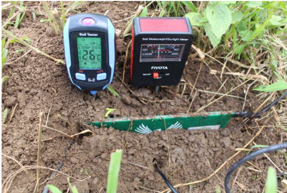
Figure 5.11: Comparative tests with commercial sensors Fivota and MIOGREN. Source: Own image of the tests performed on the parallel plate sensor.
