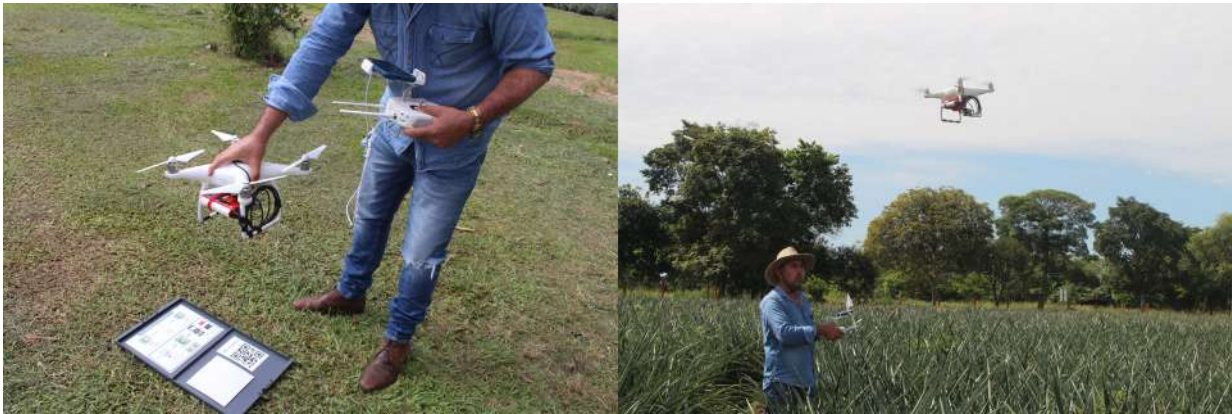
Figure 5.2: Camera calibration through the reflectance panel and stabilized flight at 12 meters altitude. Source: Own image of the equipment used in the development of the experimental design.
