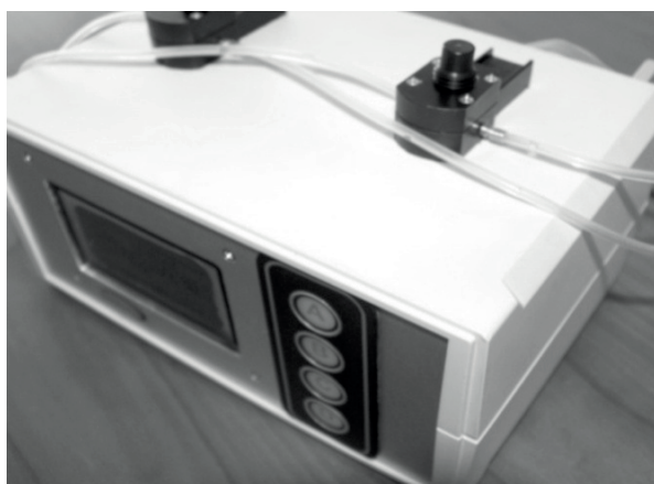
Figure 3 Portable amperometric instrument and diagram of his electronic systems
