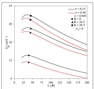
Figure 2 Variation of impurity binding energy as function of well width: magnetic-field values and indium concentrations. This is for different values of the magnetic field and for two different indium concentrations (x = 0.15 and x = 0.30).
