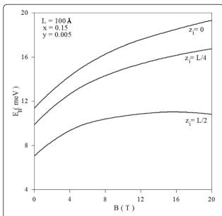
Figure 3 Variation of impurity binding energy as function of magnetic field and for two different impurity positions.
