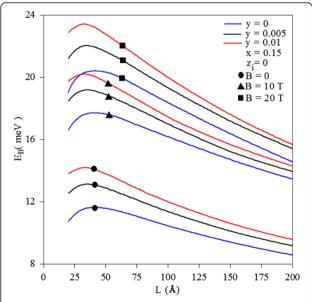
Figure 1 Variation of impurity binding energy as function of well width: magnetic-field values and nitrogen concentrations. This is for some values of the magnetic field (B = 0, 10, and 20 T) and nitrogen concentrations (y = 0, 0.005, and 0.01).
