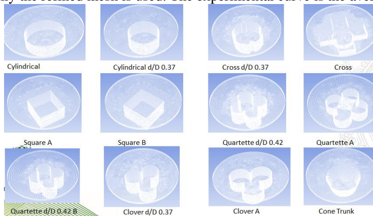
Figure 3.2 Meshes used in Fluent 3-D CFD simulations.
