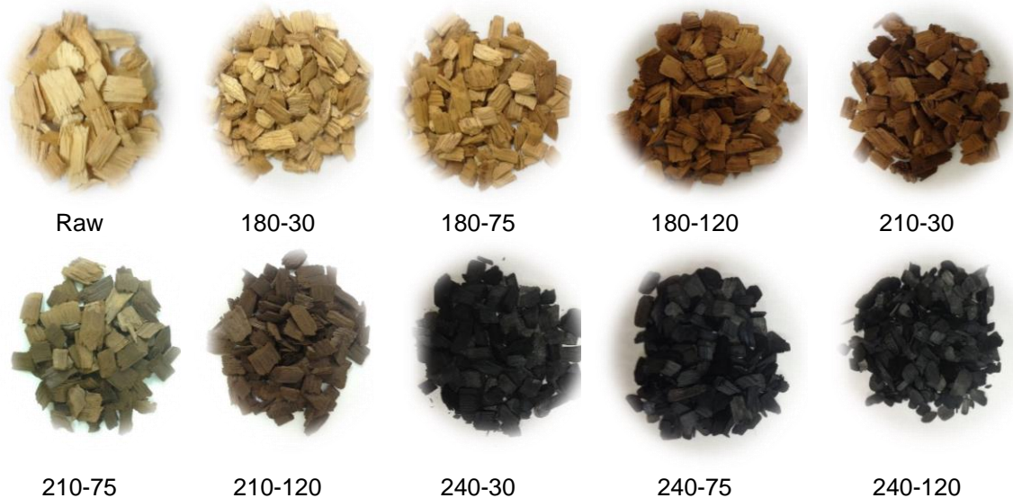
Fig. 6. Pictures of the physical changes that occurred during torrefaction of patula pine wood chips with a size range from 10 mm to 20 mm
