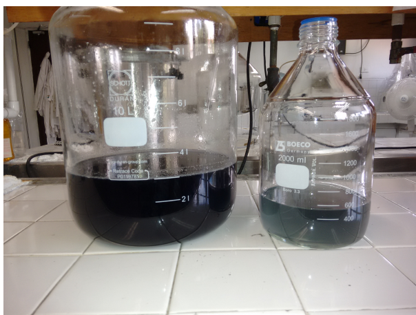
Figure 5 Close-up: wastewater, before treatment (left) and after 180 h of treatment in the 5 L reactor with Bjerkandera sp (anamorph R1) (right)
