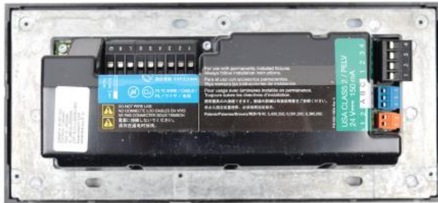
Figura 10. Wallbox power module (WPM) LQRJ-WPM-6P vista trasera.
