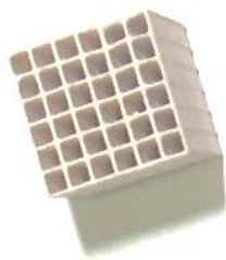
Figure 38 Image of a cordierite mini-monolith washcoated with Pd-Co/HMOR
