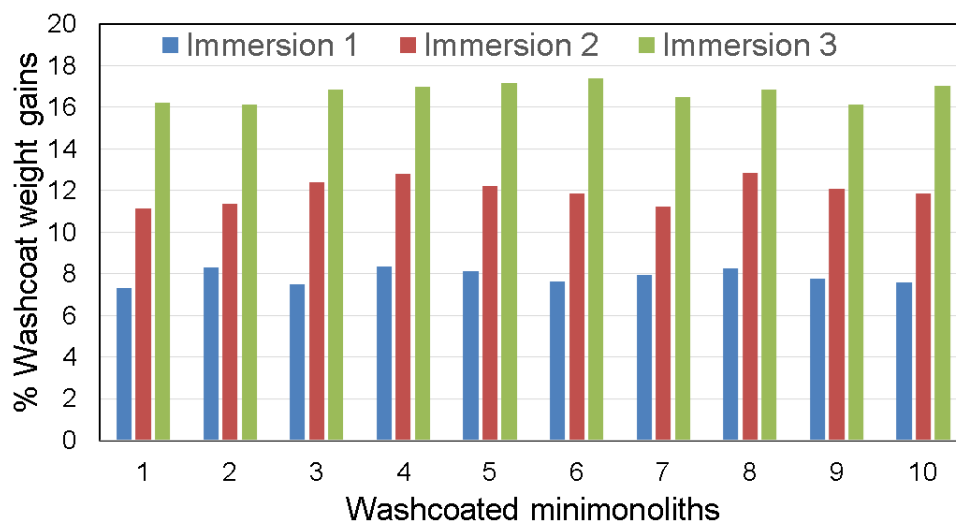
Figure 39 Washcoat loading as function of the number of immersions for each minimonolith.
