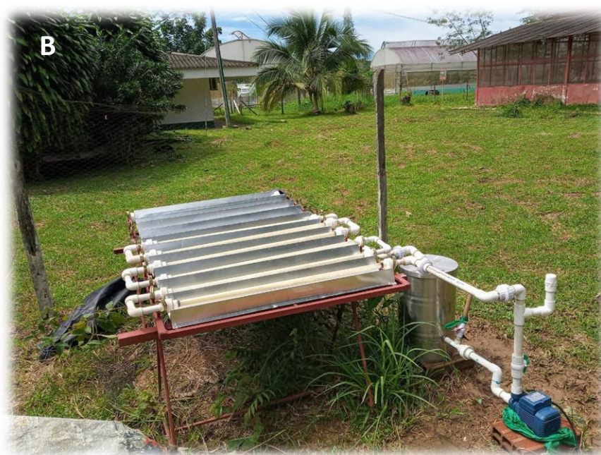
Figure 17. A. Scheme of the reactor used in the experiments at pilot-scale for the SPF process. B. Photographic record of the CPC reactor located in the Environmental Chemistry Laboratory of the Universidad de la Amazonia.
