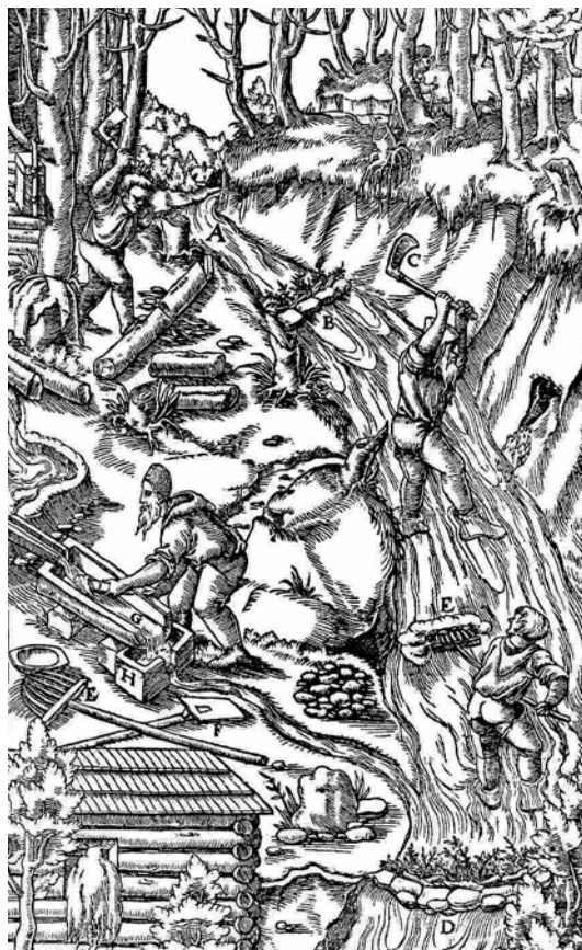
Figura 20. Grabado De re metallica (Agricola (1912 [1556]: 337). A. Stream B. Ditch. C. Mattock. D. Pieces of turf. E. Seven-pronged fork. F. Iron shovel. G. Trough. H. Another trough below it. I. Small wooden trowel. Tomado de: http://www.gutenberg.org/files/38015/38015-h/38015-h.htm .
