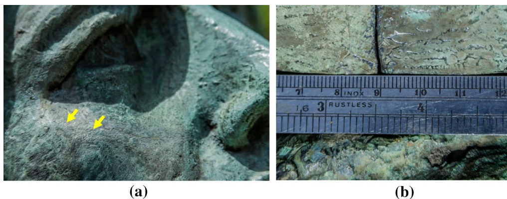
Fig. 2 Damage found on the surface of the sculpture. a Cracks. b Separation between the parts that make up the sculpture
