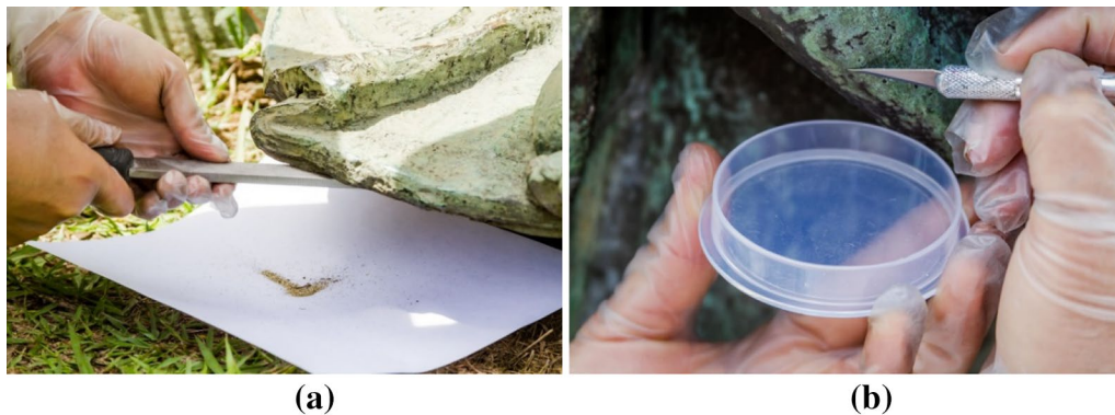
Fig. 4 Methodology for sampling. a Obtaining metal base shavings taken from the bottom of the sculpture. b Obtaining the corrosion products by mechanical cleaning with a scalpel
