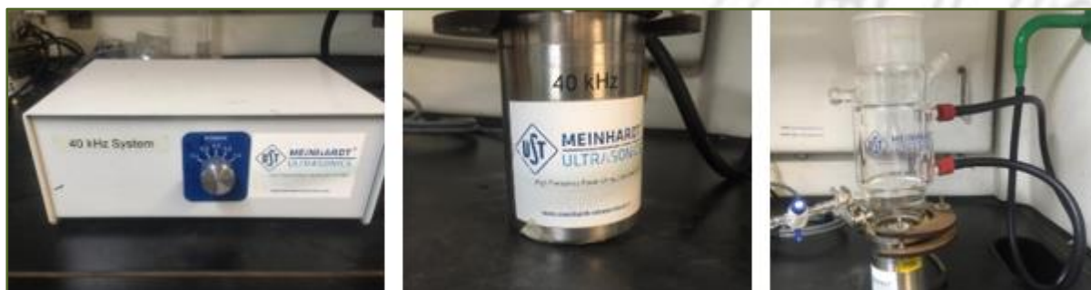
Figure 7. Sonochemical reactor (US generator-40 kHz ultrasonic transducer-glass reactor).
