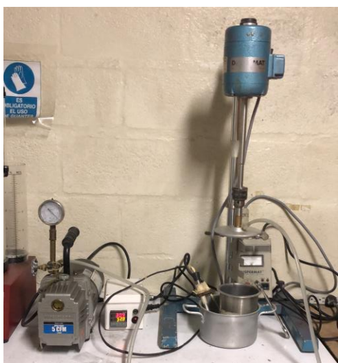
Fig. 52. Experimental setup of vacuum impregnation method using a thermostatic bath.
