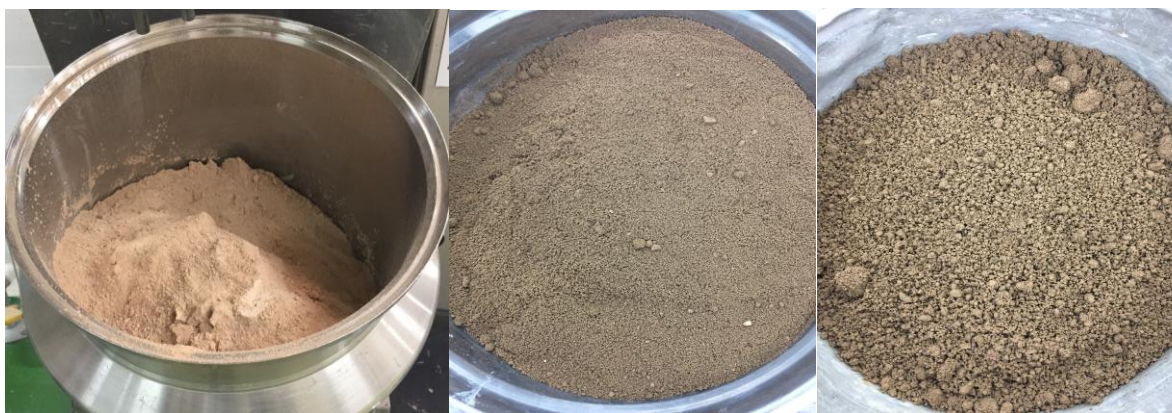
Fig. 64. Powder raw support, fine granulation and coarse granulation (from left to right).
