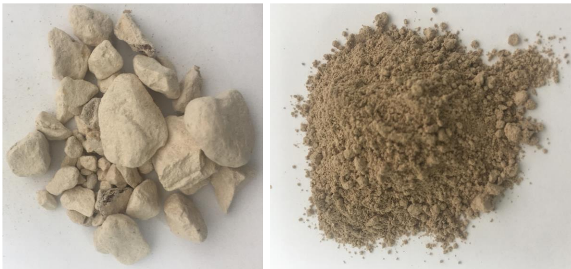
Fig. 33. Clay mineral before (left) and after (right) a grinding process.
