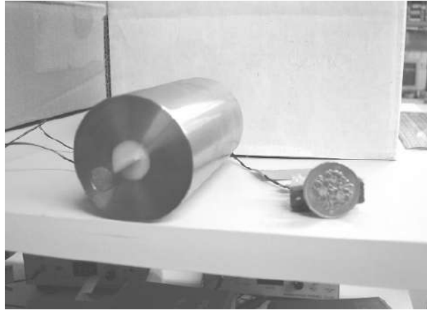
Figure 4b Set-up condition of Bender element (at pedestal)
