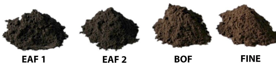
Figure 4. Steel slags subjected to crushing and grinding.
