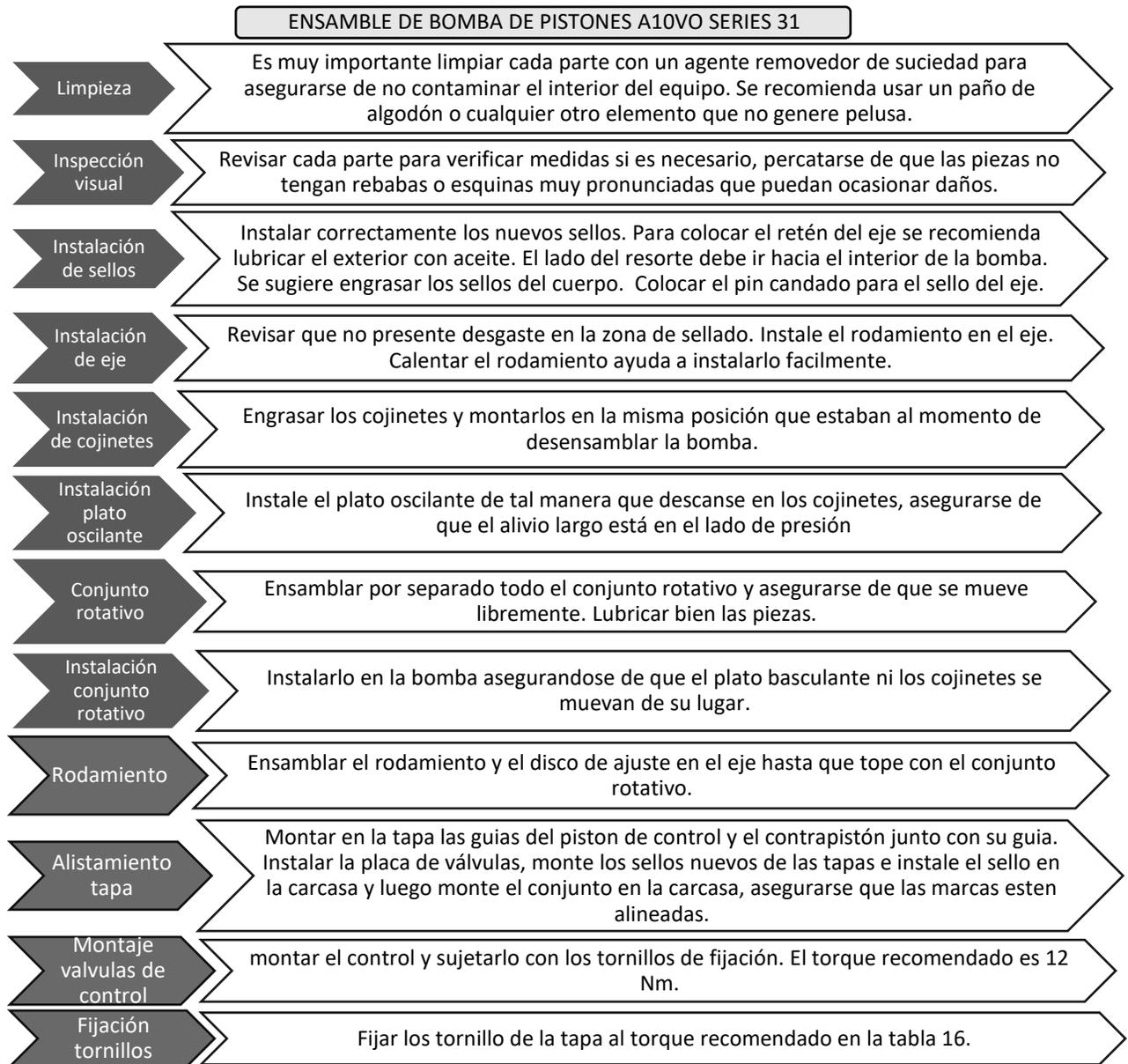
Figura 41. Ensamble de bomba de pistones Rexroth A10VO series 31
