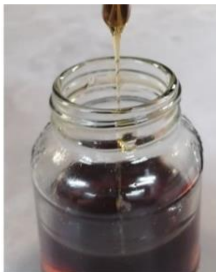
Figure 22: Carbonated sunflower oil obtained from the synthesis between ESFO and CO 2 .
