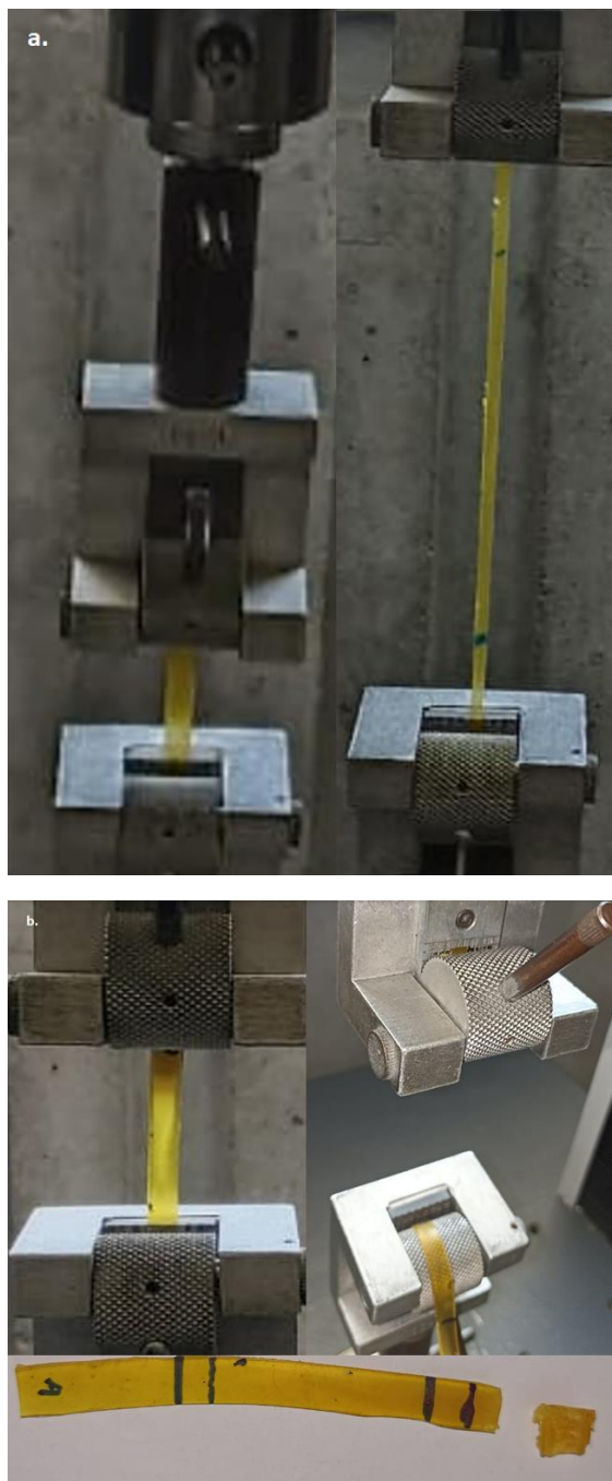
Figure 14: Images of mechanical test for a) NIPU and b) CS NIPU under tension.
