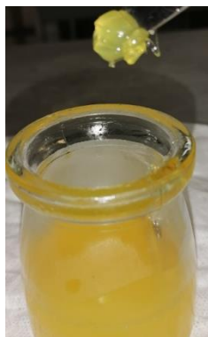
Figure 26: Polyamine polyol product obtained from the synthesis between ESFO and EDA.
