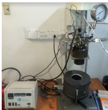
Figure 12: Experimental arrangement for the carbonation reaction.
