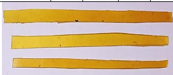
Figure 29: Polymeric NIPU3 films obtained through the reaction between CSFO and PAPO after 24 hours of oven-curing at 90 °C.
