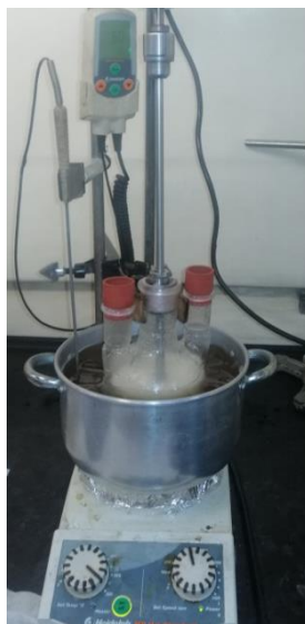
Figure 11: Experimental arrangement of the epoxidation reaction.
