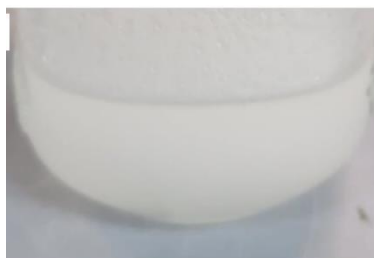
Figure 19: Viscous clear liquid oil obtained to the epoxidation of SFO reaction.
