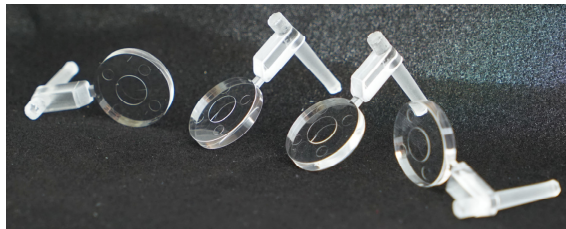
Fig. 2. Samples of polymethylmethacrylate light sword lenses (LSLs) fabricated by injection technology.
