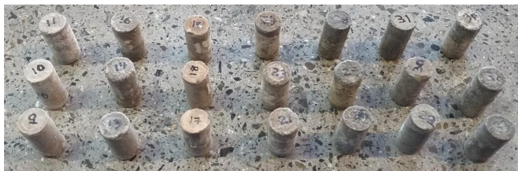
Figure 2. Alkali-activated stone wool fiber specimens with and without OPC addition.
