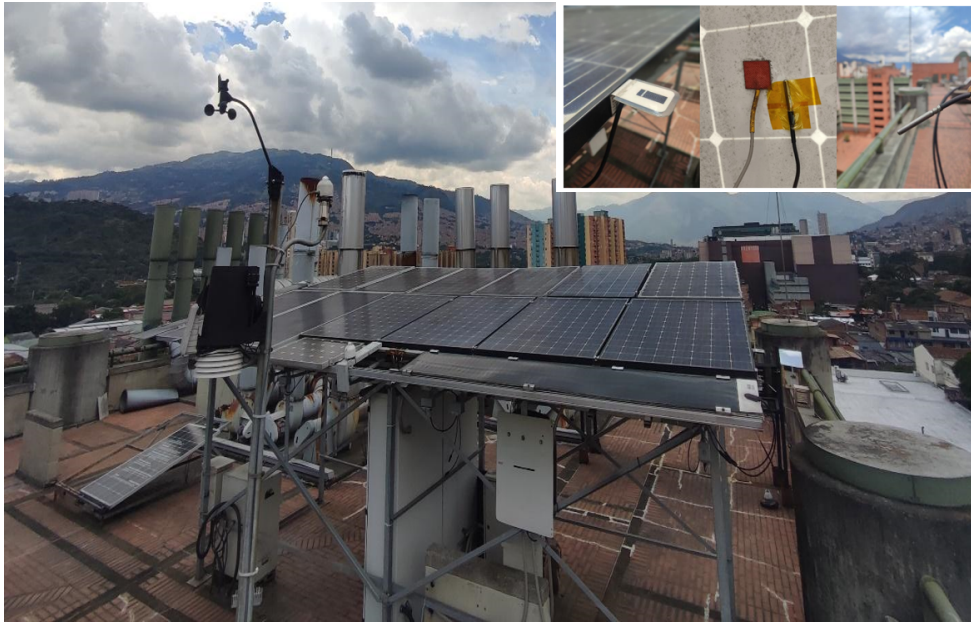
Figure 2: Solar Outdoor Laboratory for characterization of photovoltaic devices in real operating conditions, Sede de Investigación Universitaria – SIU, Universidad de Antioquia, Medellín, Colombia
