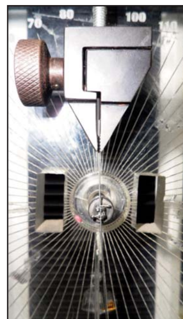
Fig. 1: An acrylic structure adapted to the INSTRON machine fixed the Upper right first bicuspid bracket, arch wire and ligature combination for the sliding test.
