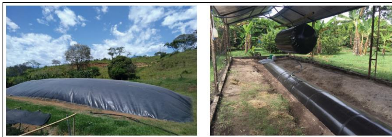
Figure 5. Plug flow reactor in pig farm commonly used in Colombia Source: PorkColombia, 2023.
