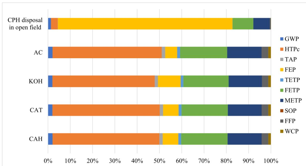
**Figure 26.** Comparative impact assessment (normalized) of value-added products and CPH disposal in open field
