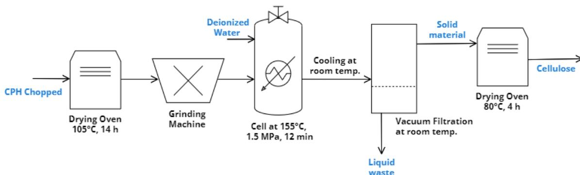
**Figure 19.** Cellulose production process through autohydrolysis (Author)
