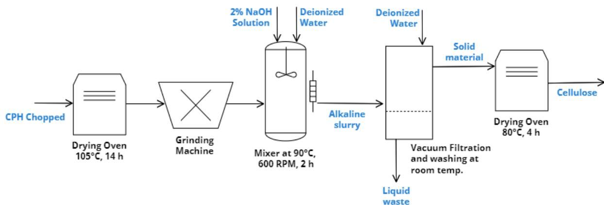
**Figure 18.** Cellulose production process through alkaline treatment (Author)
