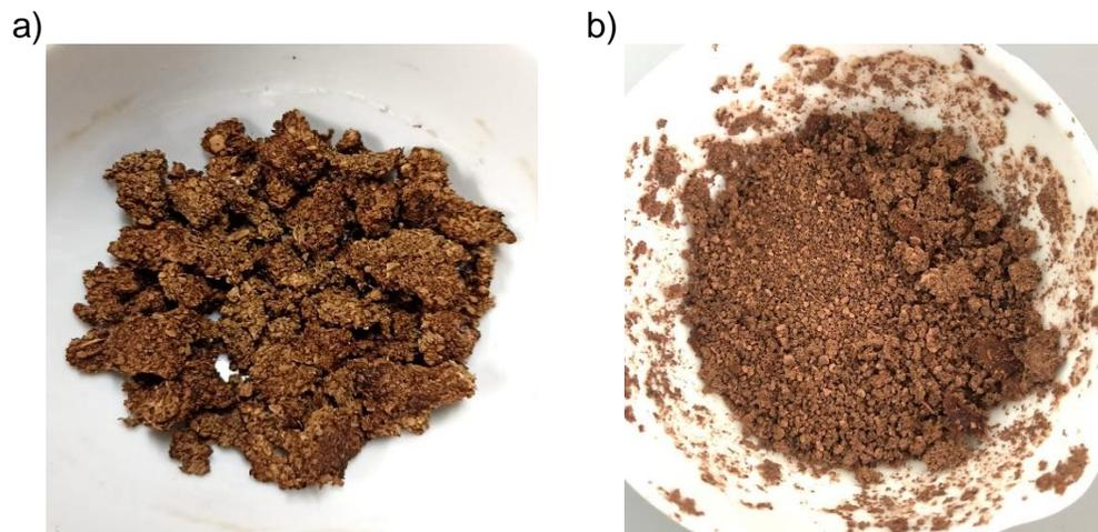
**Figure 35.** Unbleached cellulose obtained from CPH a) Cellulose by alkaline treatment, b) Cellulose by autohydrolysis (Author)
