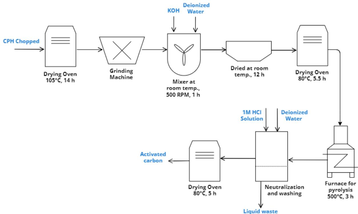
**Figure 16.** Activated carbon production process (Author)
