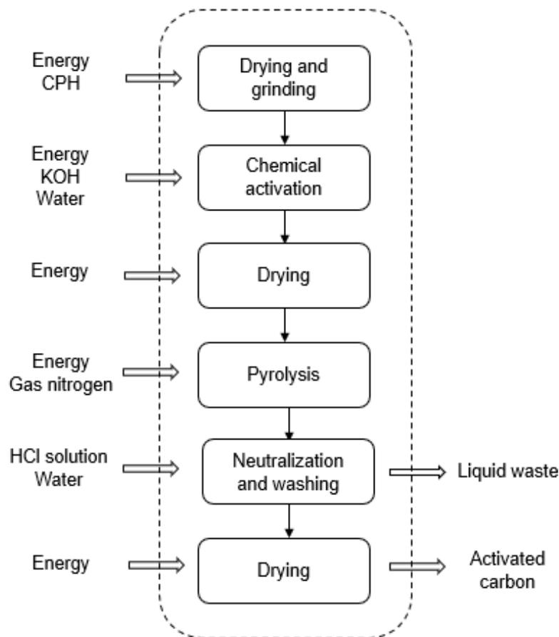
**Figure 6.** System boundaries for activated carbon production (Author)
