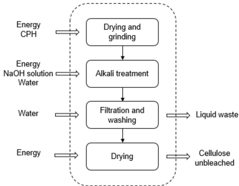
**Figure 8.** System boundaries for cellulose production by alkali treatment (CAT) (Author)
