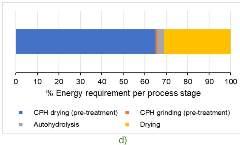
**Figure 28.** Electricity contribution per process stage to produce a) AC, b) CAT, c) CAH, d) KOH
