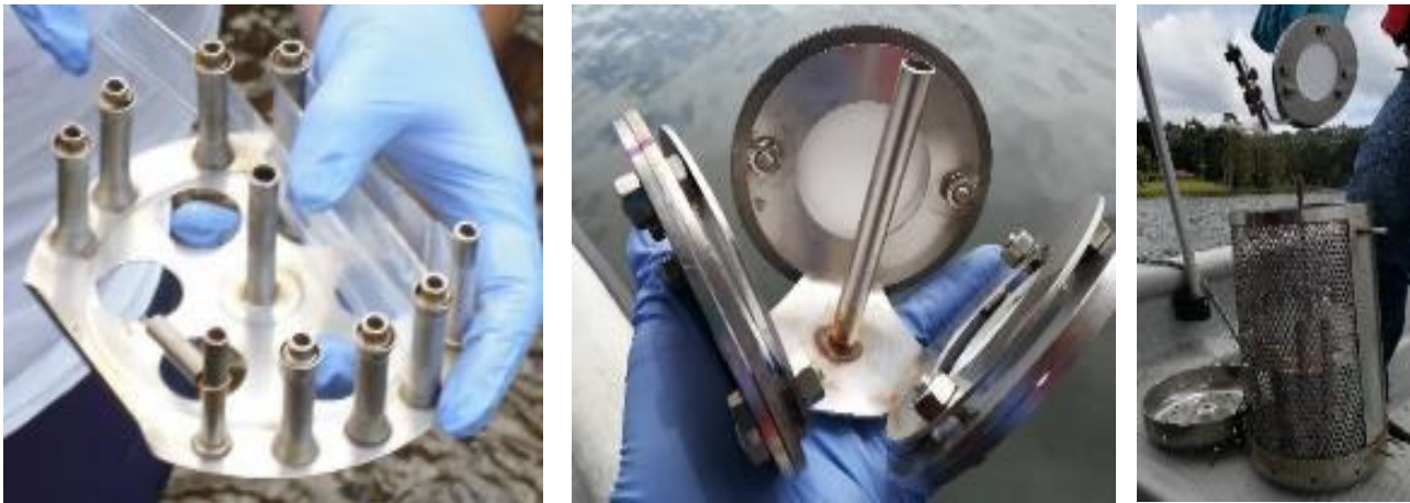
Figure 14 Arrangement of passive sampling devices in the field
