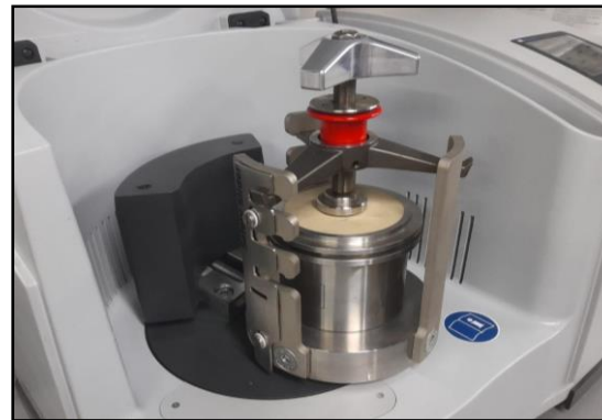
Grinding at 250 rpm for 30 min and ball ratio material 1:1 in mass
