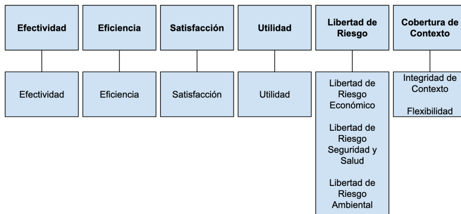
Figura 3. Modelo de Calidad de Uso ISO/IEC 25010. (ISO/IEC 25010 System and Software Quality Requirements and Evaluation [SQuaRE] — System and software quality models, 2011)
