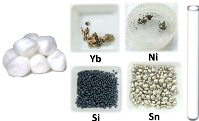
Figure 3.2: Primary elements as Yb, Ni, Si, Sn, quartz tube and quartz wool to grow \text{YbNiSi}_3 with Sn flux.
