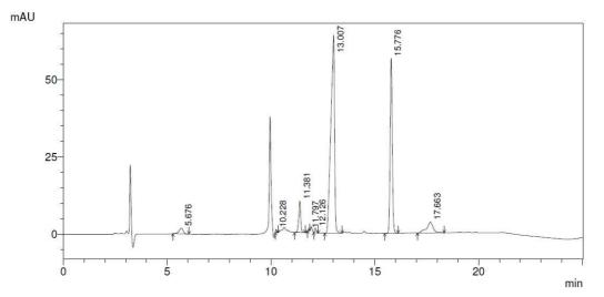
Figure 2: Chromatographic profile of photodegraded solution of hybrid 19. C18 column and water pH 3.0: acetonitrile as mobile phase under gradient
