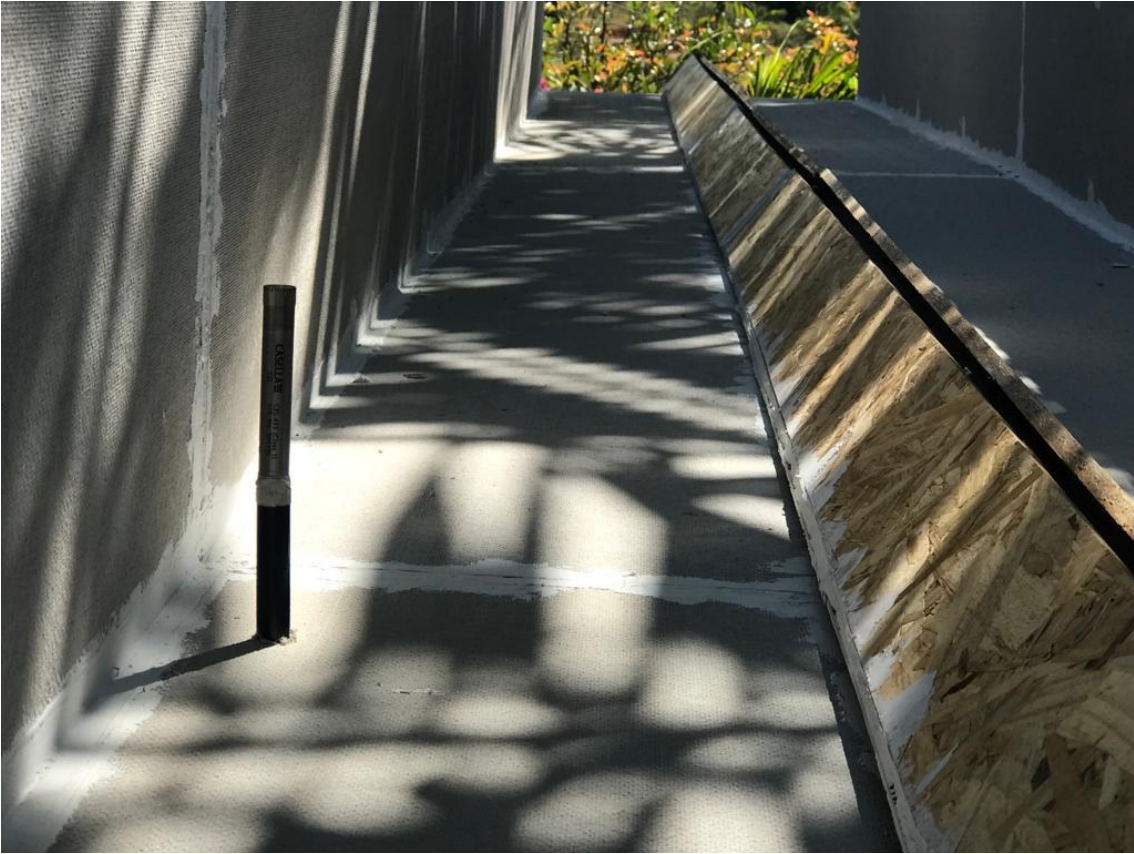
Fig. 46 Measurement microphone on the scale model. (Taken from own source).
