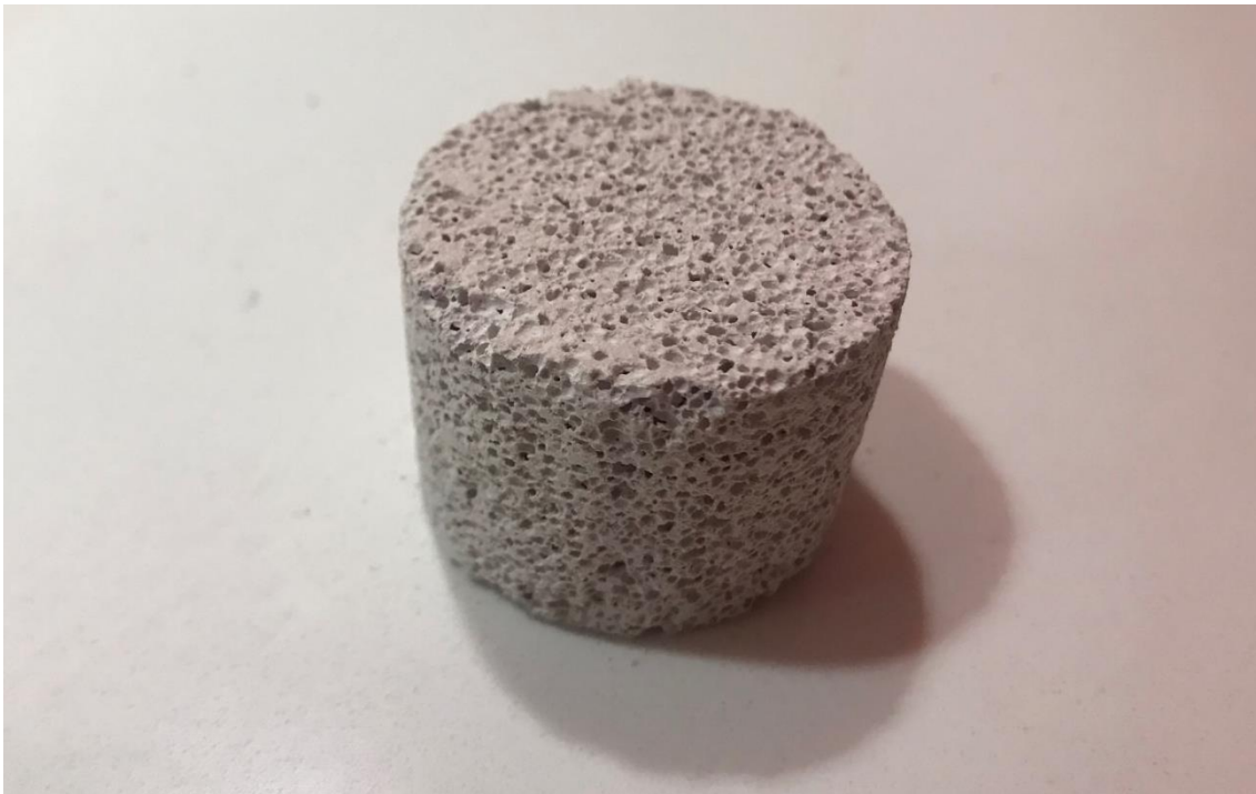
Fig. 54 Pumice stone sample (3.5 cm high and 4 cm in diameter). (Taken from own source).
