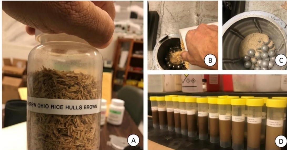
Fig. 24 Grinding process. A) Rice husk used for milling. B) Dumping of the rice husk in the ball mill. C) Grinding after 12 hours. D) Rice husk nanoparticle samples with deionized water and PVP. (Taken from own source).
