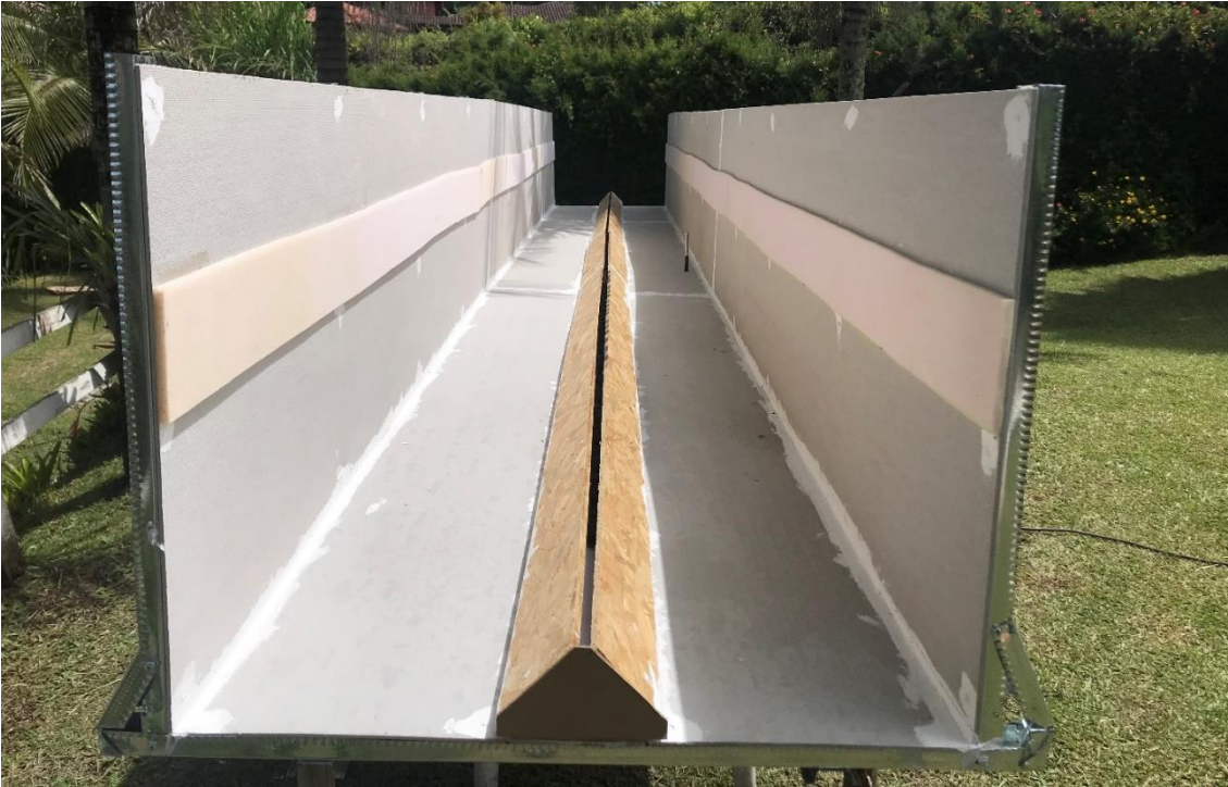
Fig. 52 Scale model (1:10) with continuous absorbing hard foam, alloy steel structure, fiber-cement plates, line array of tweeters with acoustic box, and measurement microphone. (Taken from own source).
