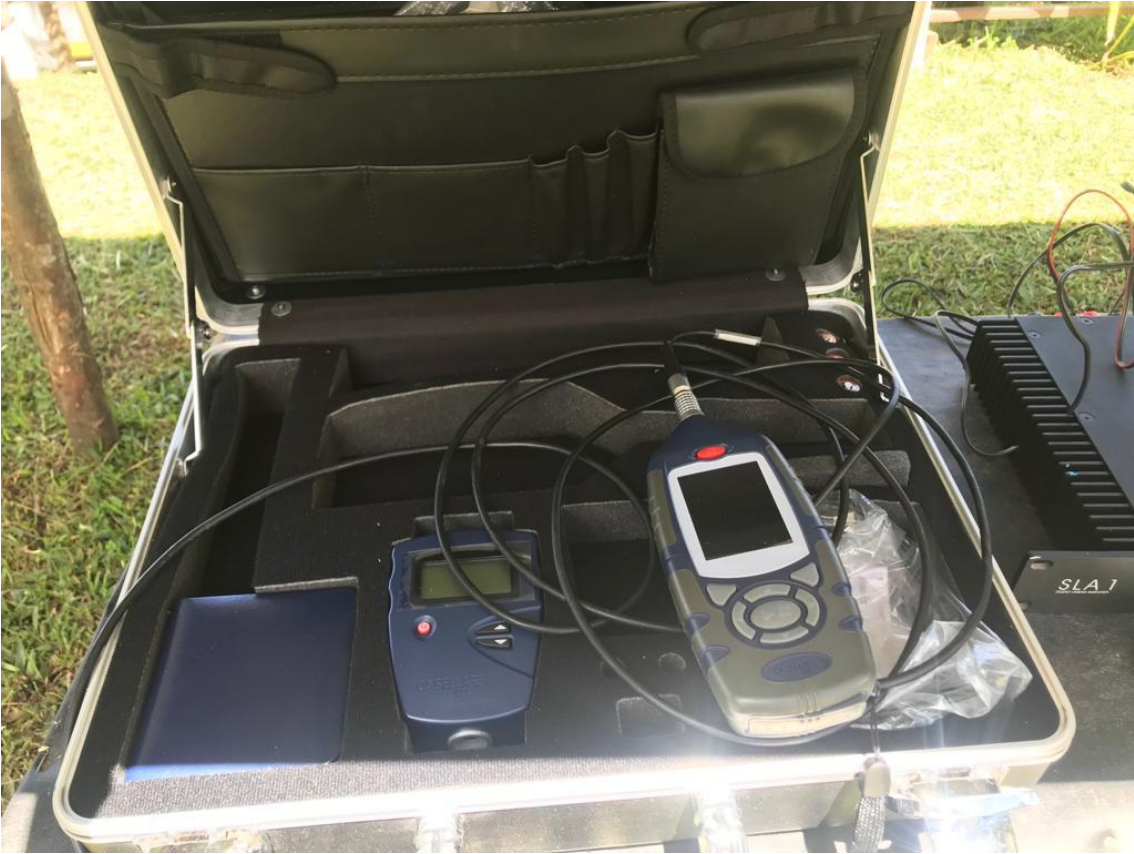
Fig. 44 Detail of the sound level meter used for the measurement. (Taken from own source).
