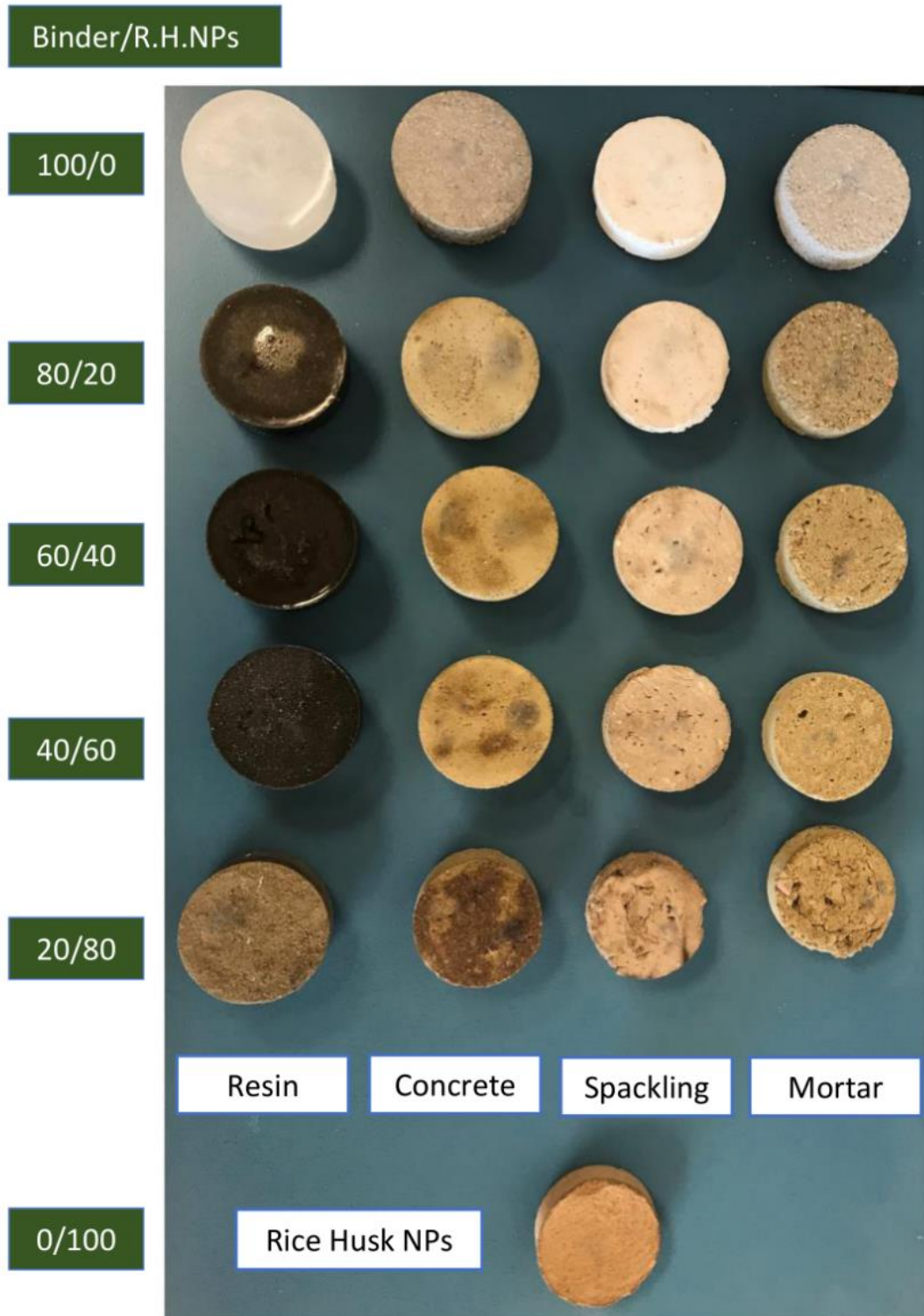
Fig. 26 Experiment design of samples analyzed in the impedance tube. From left to right (Epoxy Resin, Concrete Mix, Vinyl Spackling, Mortar Mix). From top to bottom Composite/Rice Husk NPs (100/0, 80/20, 60/40, 40/60, 20/80, 0/100). (Taken from own source).
