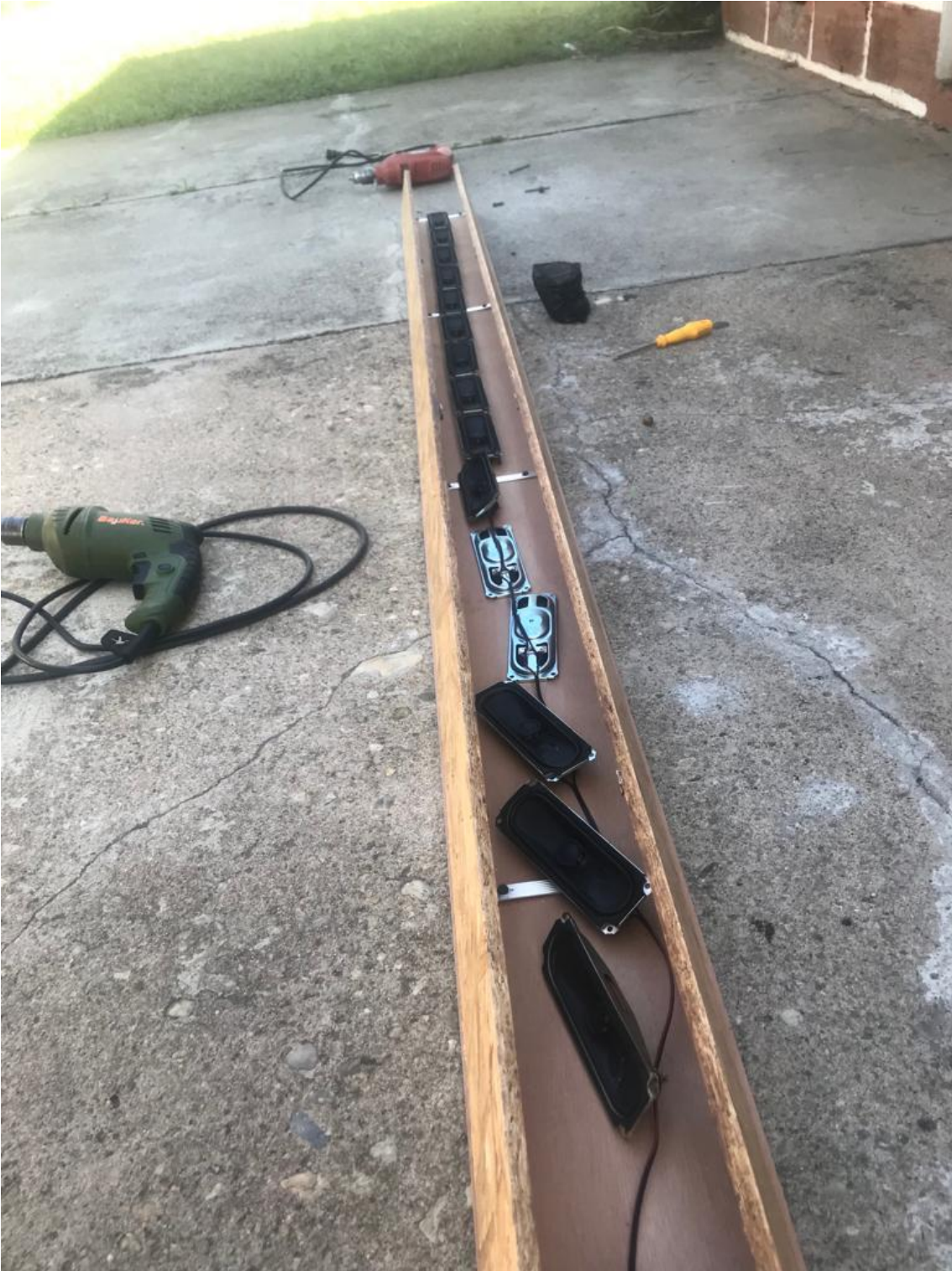
Fig. 42 Speaker assembly inside the baffle. (Taken from own source).
