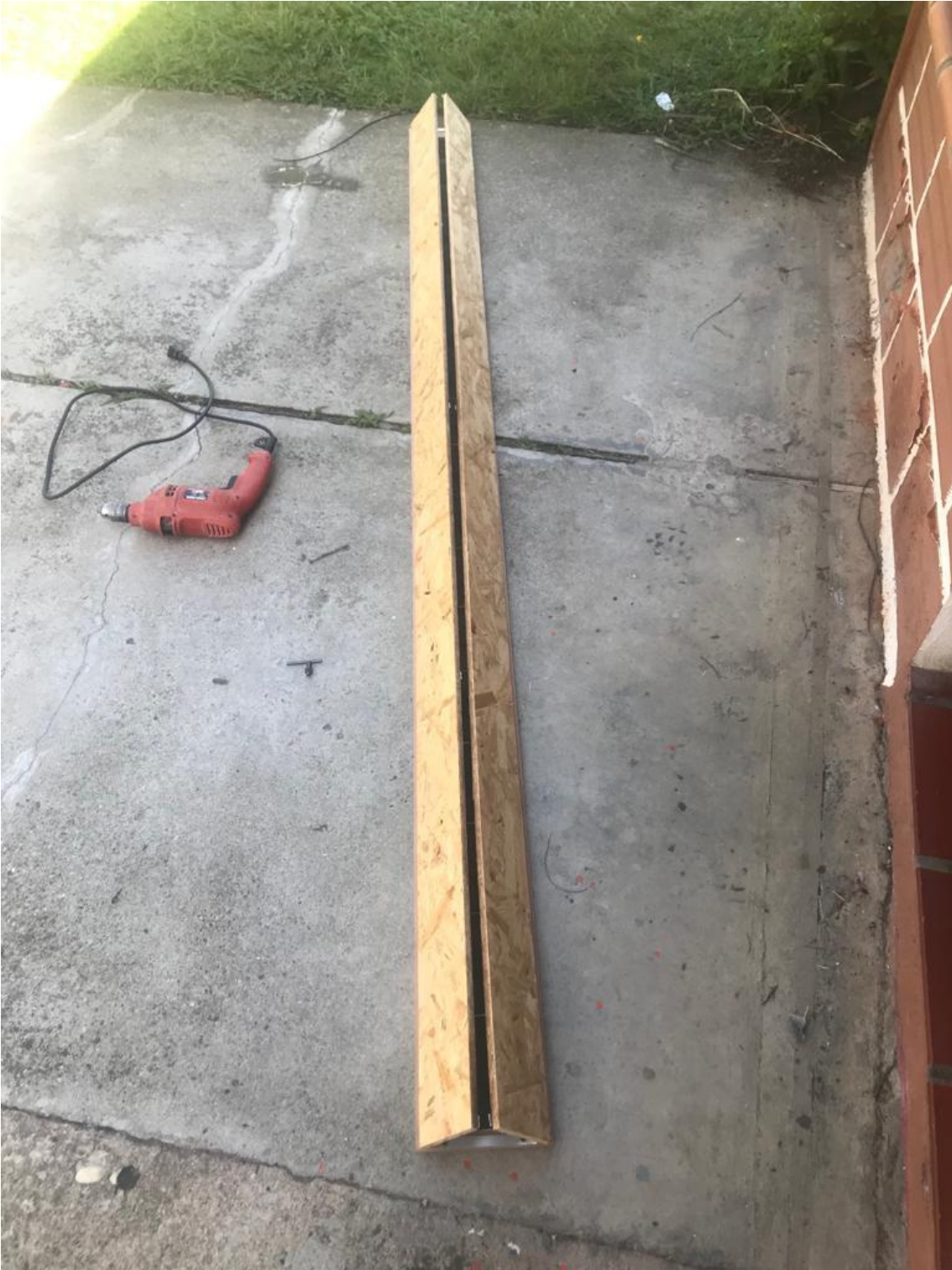
Fig. 43 Baffle with opening at the top for sound radiation. (Taken from own source).
