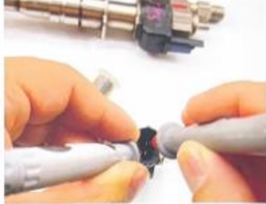
6. Measuring the plug connections of fuel injectors
