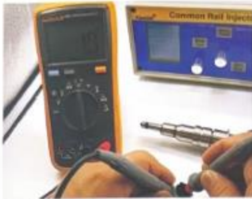
5. Use multimeter to measure the resistance of the injector
