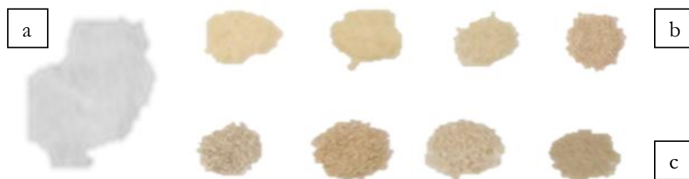
Figure 37 Change of color in zeolites 4A used. (a) fresh zeolite 4A; (b) After methanol adsorption; (c) After CO 2 adsorption .
