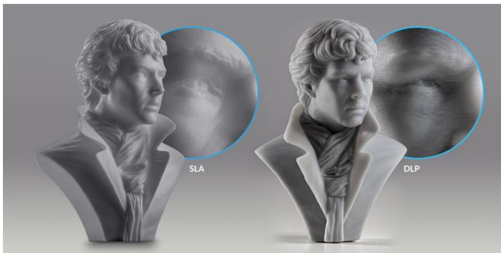
Figure 1. Resolution difference between SLA and DLP technologies. Taken from [5].
