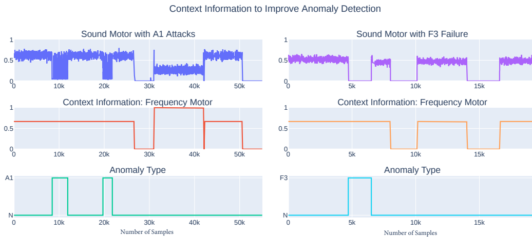
Figure 5.13: Context information. By incorporating motor data into the Industrial Internet of Things (IIoT) dataset, it becomes possible to distinguish between normal and abnormal behavior.
