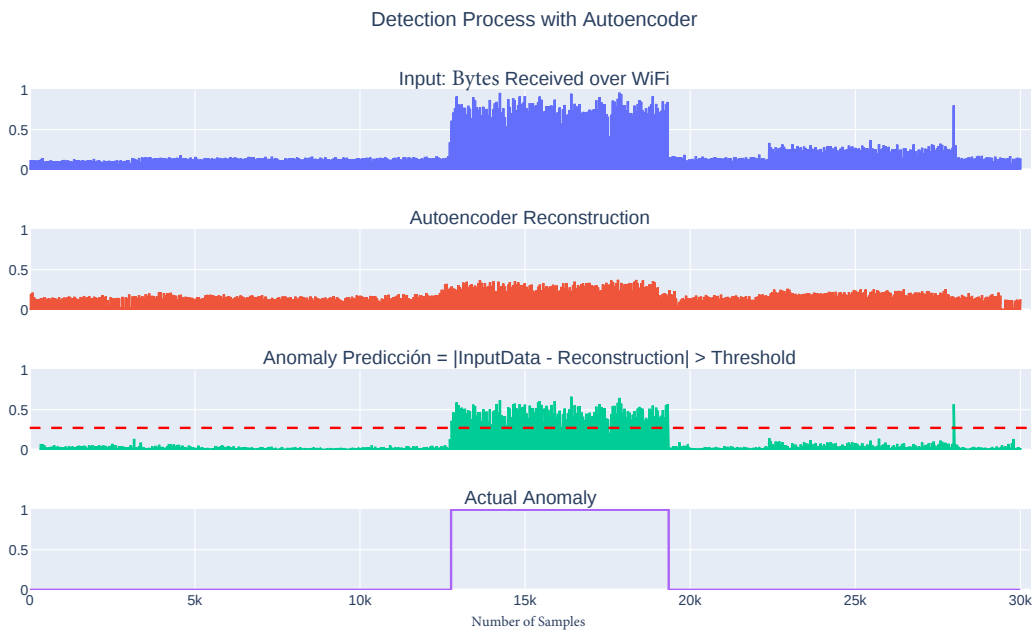
Figure 5.15: Anomaly Prediction with Autoencoder. Any sample above the threshold value is labeled as an anomaly.
