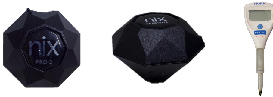
Fig. 1. Portable devices used for data acquisition: Nix Pro 2 and Nix Spectro 2 spectrophotometers (left and center) for colorimetry and visible spectroscopy, and Hanna Foodcare pH meter (right) for ultimate pH measurement in beef carcasses.
