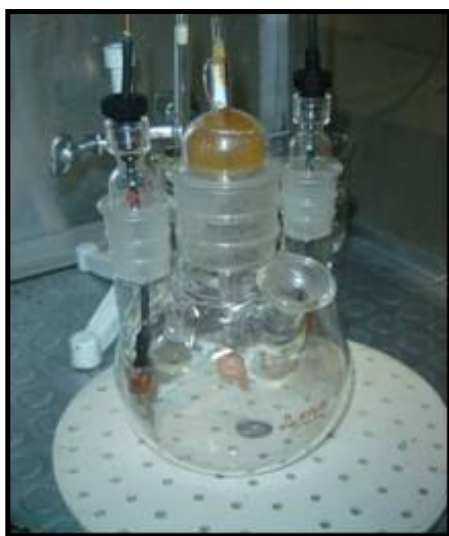
Figure 8. Electrochemical cell used for the potentiodynamic reductions.
